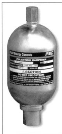
Figure 7. Appendage type 60 in 3 1,500 psi stainless steel pulsation dampener with threaded fluid port.
